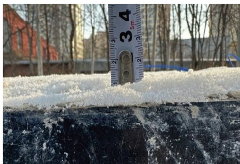
Fig.22 Snow thickness on pavement surface area
