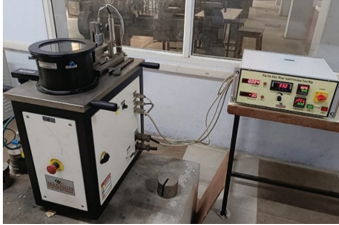
Fig.2 Pin-on-disc wear and friction tester
