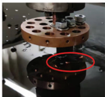
Fig. 6 Three-electrode discharging simultaneously in machining
