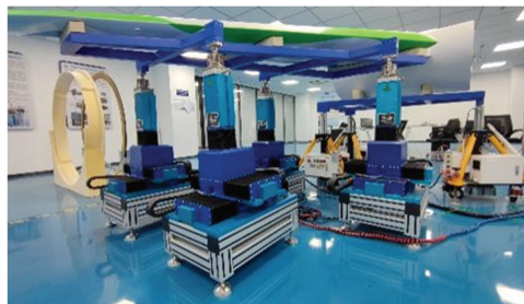
Fig. 4 Multi-point array support experimental system
