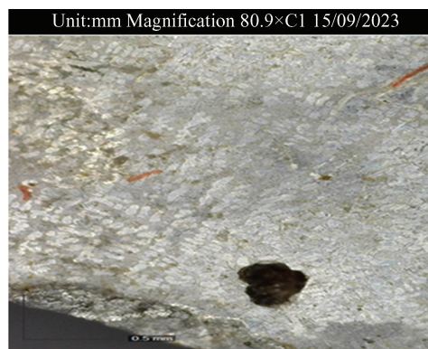
(b) Microscopic image of AlSi10Mg heat sink without heat treatment
