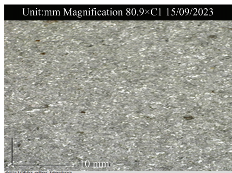
(b) Microscopic image of heat sink after abrasive blasting at 0.15 MPa pressure
