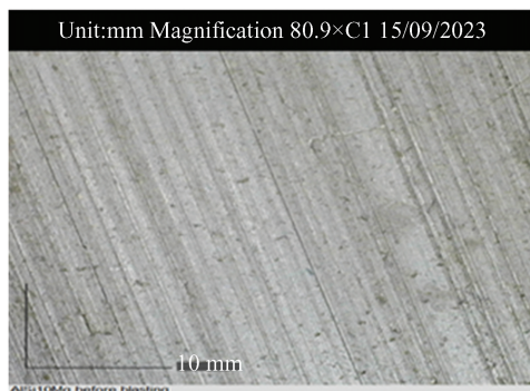
(a) Microscopic image of heat sink before abrasive blasting
