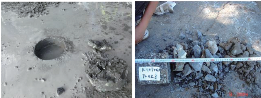
(a) 芯样破损高度大于20% (b) 芯样松散
