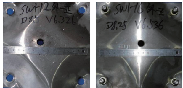
(a) SW1-12 防护屏 ( v=6.326 km/s, d_p=0.850 cm) (b) SW1-16 防护屏 ( v=6.536 km/s, d_p=0.825 cm)
