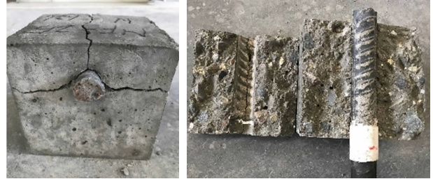
(a) NF-1-1: 劈裂破坏
