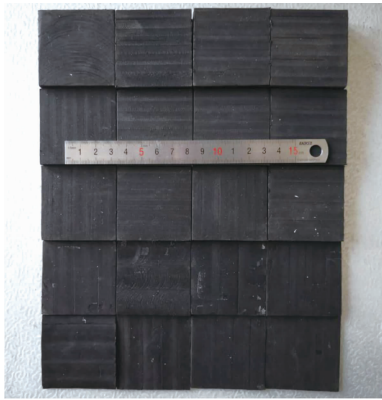
图 4 落锤实验所用试样 Fig. 4 Samples for drop hammer test
