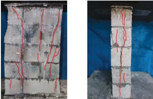
图 5 试件典型破坏形态 Fig.5 Typical failure patterns of the specimens
